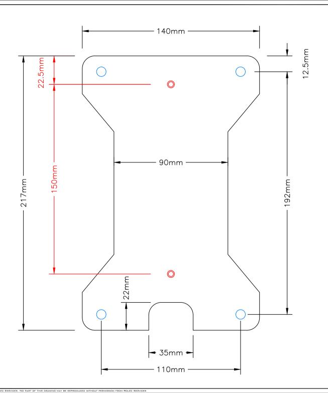
WALLPOD BACK PLATE TO FIT ZURA POST (217MM x 140MM) MATERIAL: 2MM CR4 MILD STEEL P/C BLACK
